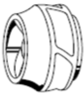
Closed (shrouded) mixed flow impeller *)
