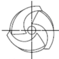
Closed (shrouded) mixed flow impeller *)
