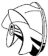
Open (unshrouded) mixed flow impeller
