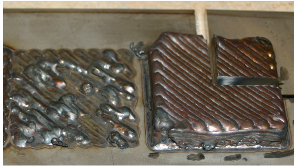
Figure 11: Deposit without continuous process control (left) and with continuous process control (right).
