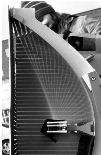
Figure 4.17 An example of optical ray tracing on Solar8, with 0° angle of incidence and a 60 mm thick absorber (Photo by Håkan Håkansson)
