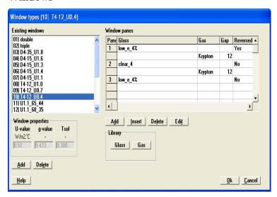
When a window is selected a calculation of the U-value, g-value and Tsol-value for the window package is done. g-value stands for the total solar energy transmission and Tsol for the primary solar energy transmission. The calculation is done according to the standard ISO 15099.
