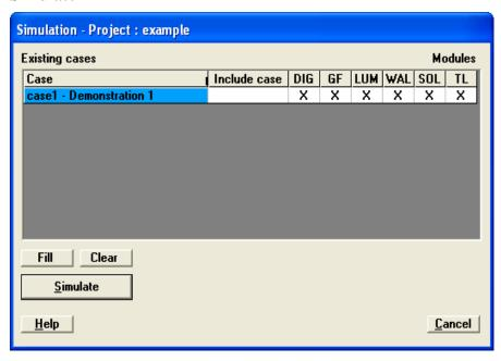
The DEROB-LTH program is built up of six different calculation modules. The models are automatically checked. A complete simulation includes all modules. It's however possible for an experienced user to manually select modules to be run. The list 'Existing cases' contains one or more cases (building models) located in the opened design project. One or more of these can be checked to be simulated.
