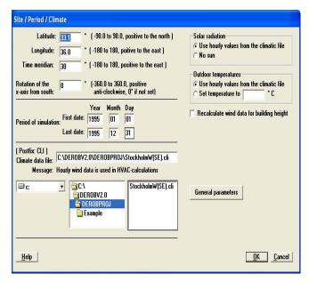
The climatic data file should include data for wind-speed and wind-direction to be used for the calculations of natural ventilation. It's however working even if these data are missing, but with loss of accuracy in the results.
