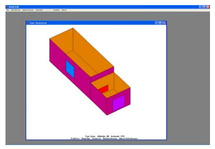
With this function it's possible to rotate the building in all directions and visibly remove arbitrary surfaces to be able to look into the building. The 3-D view function is especially useful in the build-up of the building geometry. Then it's important to check that surfaces are located in the correct position and orientated as intended.
