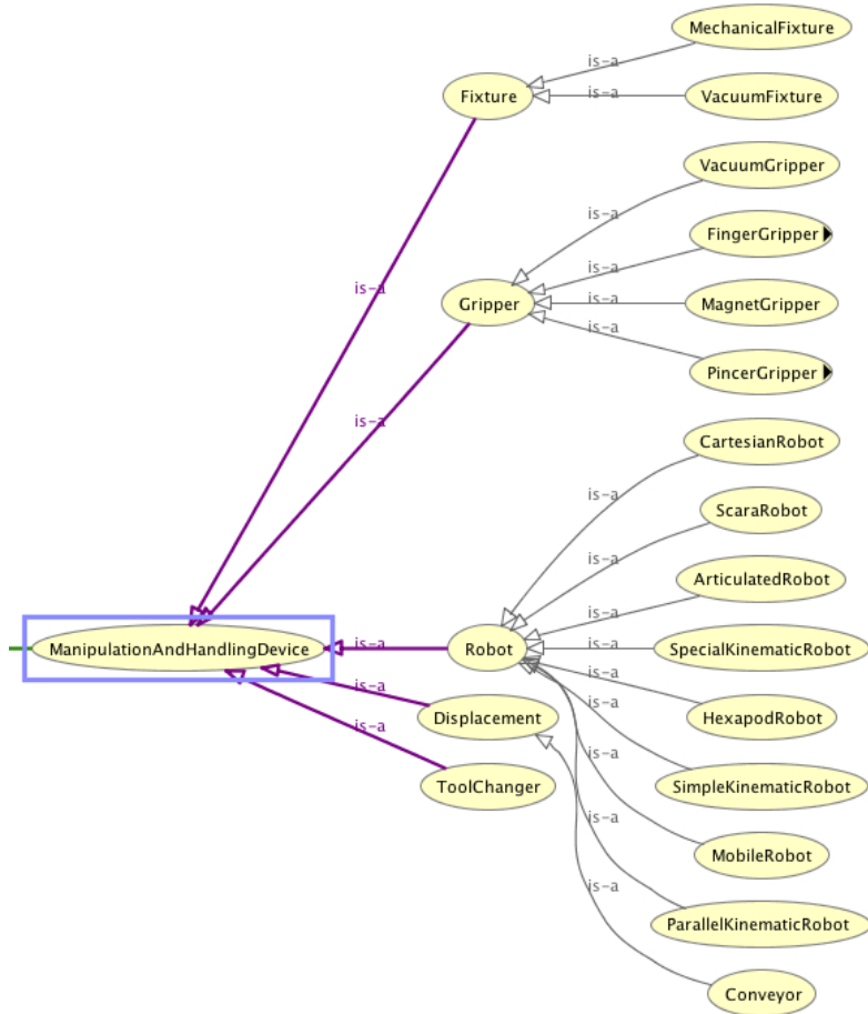
Figure 3: Manipulation and handling devices, as defined by SIARAS ontology.
