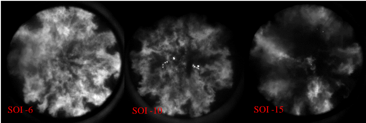
Figure 10: Combustion for different SOI's. As expected, earlier injection timings will have more mixing time and exhibit lower intensity when combusting.
