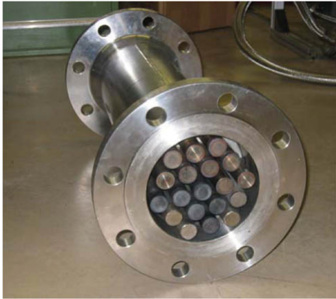
Figure 3: Shell and tube configuration. The PCM is located in the cylindrical capsules (source: German Aerospace Center (DLR) ( http://spie.org/x8476.xml?pf=true&ArticleID=x8476 )).
