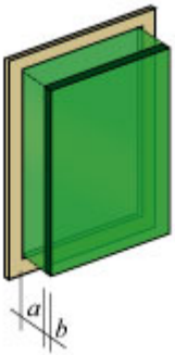
Fig.5.3.2 A schematic picture of a shutter, the new type of external sunshade.
