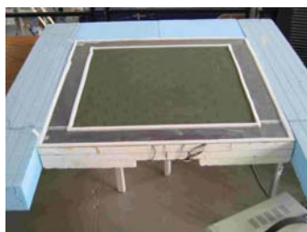
Fig. 4.2.5 The measuring area and the guarded ring.
