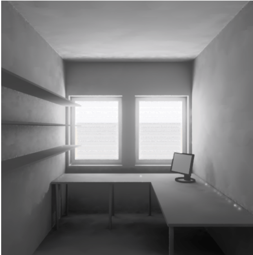
Figure 4.27 Image simulated in Radiance for the solar altitude in June at 12.00 true solar time
