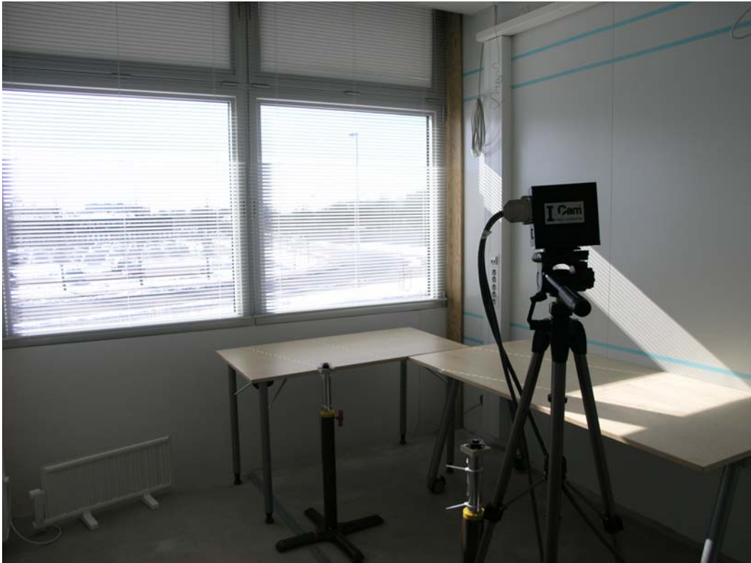
Figure 4.1 During the set-up phase, it became obvious that the angle difference between the upper and lower sections was too great, allowing direct solar radiation onto the work surface. This was corrected before the measurements started. (Photograph: Thore Sonesson).
