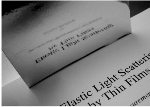
Fig. 6. Visual appearance of the Al-on-steel reflector: a photograph of a thesis on light scattering, reflected in the solar reflector laminate.
