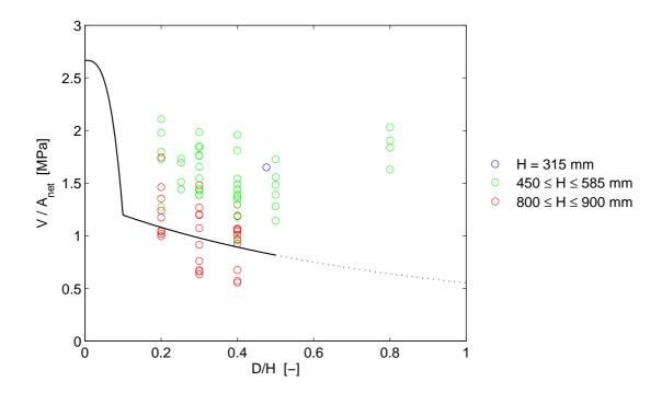
Figure 5.10: Characteristic capacity  $V_k/A_{net}$  according to Limträhandbok method 1 compared to  $V_c/A_{net}$  for experimental tests on circular holes  $(D = \phi)$ .  $V_k/A_{net}$  valid for all beam heights H and based on beam width T = 90 mm.
