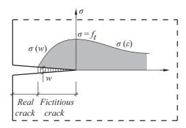
Figure 3.5: Illustration of stresses in FCM [11].
