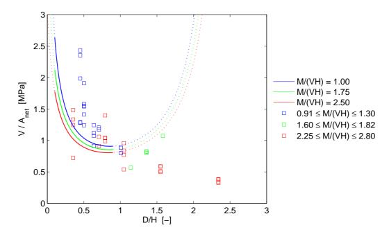
Figure 5.21: Characteristic capacity  $V_k/A_{net}$  according to DIN 1052:2004 and DIN 1052:1999 for different bending moment to shear force ratio M/(VH) compared to  $V_c/A_{net}$  for experimental tests on rectangular holes  $(D = \sqrt{a^2 + b^2})$ .  $V_k/A_{net}$  valid for all beam heights H and based on hole side length ratio a/b = 2.0.
