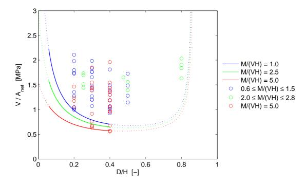
Figure 5.19: Characteristic capacity  $V_k/A_{net}$  according to DIN 1052:1999 for different bending moment to shear force ratio M/(VH) compared to  $V_c/A_{net}$  for experimental tests on circular holes  $(D = \phi)$ .  $V_k/A_{net}$  valid for all beam heights H.
