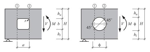
Figure 5.3: Notations for rectangular and circular holes for design according to DIN 1052:2004-08.
