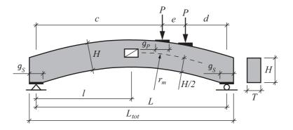
Figure 2.5: Test setup 5.
