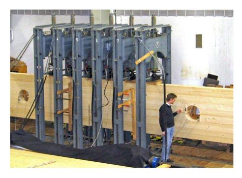
Figure 1.2: Full scale test glulam beam with holes, MPA Stuttgart [32]
