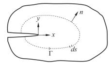
Figure 3.4: Notations used in J-integral method.
