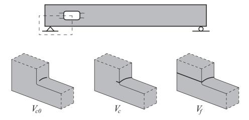
Figure 2.7: Illustration of crack patterns for crack location lb at load levels  $V_{c0}$ ,  $V_c$  and  $V_f$ . The same crack patterns are valid for crack locations lt, rb and rt.
