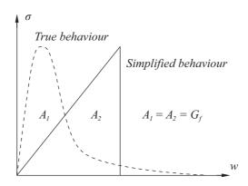
Figure 3.6: Illustration of true and simplified stress-deformation relationship [7].
