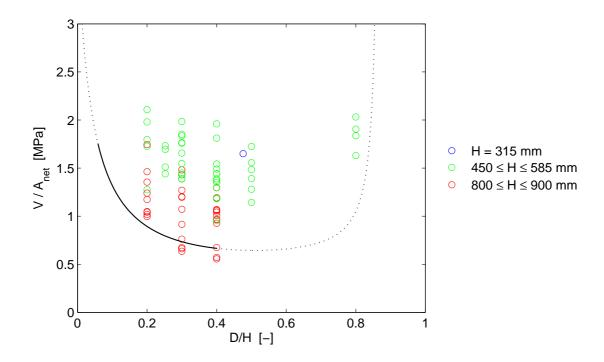
Figure 5.18: Characteristic capacity  $V_k/A_{net}$  according to DIN 1052:1999 compared to  $V_c/A_{net}$  for experimental tests on circular holes  $(D = \phi)$ .  $V_k/A_{net}$  valid for all beam heights H and based on bending moment to shear force ratio M/(VH) = 2.0.
