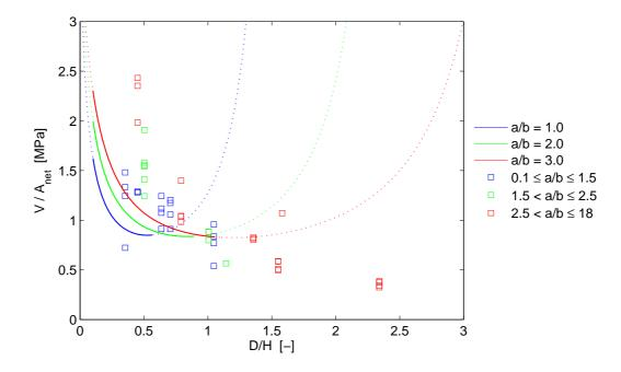
Figure 5.22: Characteristic capacity  $V_k/A_{net}$  according to DIN 1052:2004 and DIN 1052:1999 for different hole side ratios a/b compared to  $V_c/A_{net}$  for experimental tests on rectangular holes ( $D = \sqrt{a^2 + b^2}$ ).  $V_k/A_{net}$  valid for all beam heights H and based on bending moment to shear force ratio M/(VH) = 2.0.
