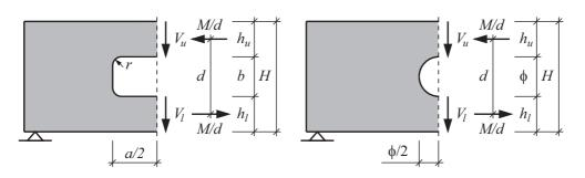
Figure 5.1: Notations for design according Method 1, Swedish Limträhandbok.
