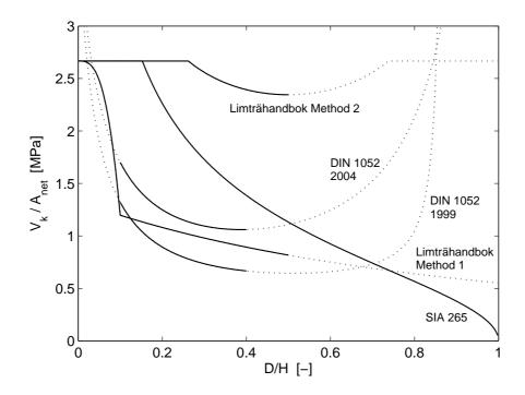
Figure 5.8: Characteristic capacity  $V_k/A_{net}$  according to codes for beams with cross section  $H \times T = 500 \times 90 \text{ mm}^2$  and with circular holes  $(D = \phi)$ . The curves for DIN 1052 are based on M/(VH) = 2.0.
