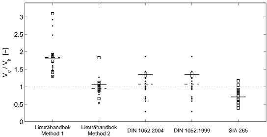
Figure 5.7: Ratio between mean crack load  $V_c$  from experimental tests on test series with rectangular holes and characteristic capacity  $V_k$  according to codes.
