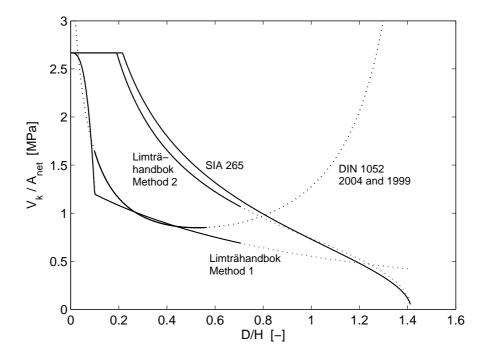
Figure 5.9: Characteristic capacity  $V_k/A_{net}$  according to codes for beams with cross section  $H \times T = 500 \times 90 \, \text{mm}^2$  and with quadratic holes  $(D = \sqrt{a^2 + b^2}, \, a = b)$ . The curves for DIN 1052 are based on M/(VH) = 2.0.
