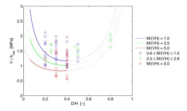
Figure 5.17: Characteristic capacity  $V_k/A_{net}$  according to DIN 1052:2004 for different bending moment to shear force ratio M/(VH) compared to  $V_c/A_{net}$  for experimental tests on circular holes  $(D = \phi)$ .  $V_k/A_{net}$  valid for all beam heights H.
