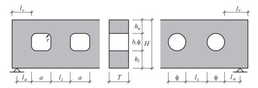
Figure 5.5: Notations for regulations concerning hole geometry and placement.
