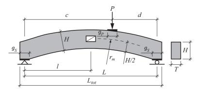
Figure 2.4: Test setup 4.
