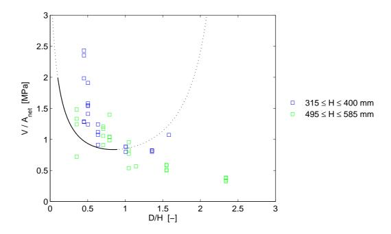
Figure 5.20: Characteristic capacity  $V_k/A_{net}$  according to DIN 1052:2004 and DIN 1052:1999 compared to  $V_c/A_{net}$  for experimental tests on rectangular holes (D =  $\sqrt{a^2 + b^2}$ ).  $V_k/A_{net}$  valid for all beam heights H and based on bending moment to shear force ratio M/(VH) = 2.0 and on hole side length ratio a/b = 2.0.
