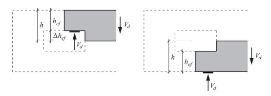
Figure 5.4: Notations for design according to SIA, tension perpendicular to grain (left) and compression perpendicular to grain (right).
