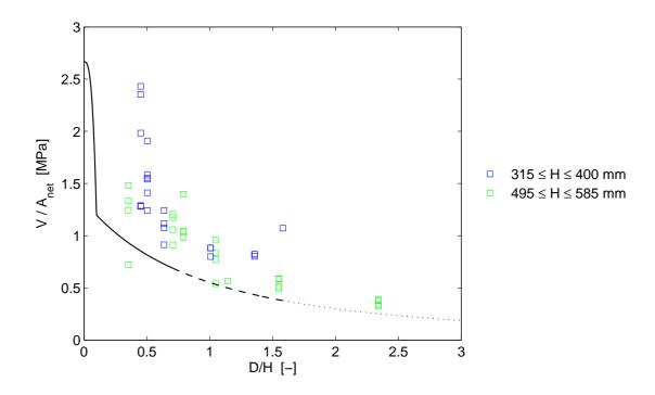
Figure 5.12: Characteristic capacity  $V_k/A_{net}$  according to Limträhandbok method 1 compared to  $V_c/A_{net}$  for experimental tests on rectangular holes  $(D = \sqrt{a^2 + b^2})$ .  $V_k/A_{net}$  valid for all beam heights H and based on beam width T = 90 mm.
