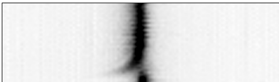
Fig. A17. Laser-induced coherent strain wave propagation into an InSb crystal.
