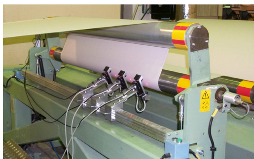
Fig. C9. The crepe-wrinkle detector mounted in a rewinder at a paper mill (left). Typical response due to a large crepe wrinkle (right).
